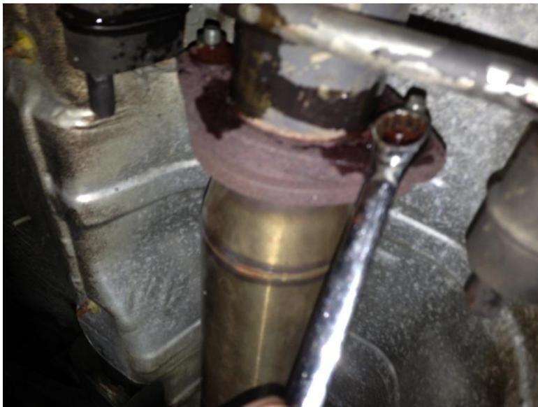
4. Carefully remove remainder of previous exhaust system and set aside.
