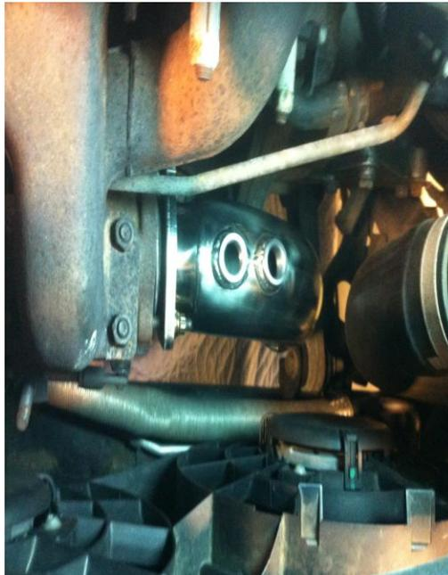
8. Install resonator pipe by placing an exhaust clamp over the pipe prior to its connection and then sliding the pipe forward into the exhaust hangers and connecting it with the downpipe. Repeat this process as you move to the rear of the car ensuring all connections are aligned properly and seated.
