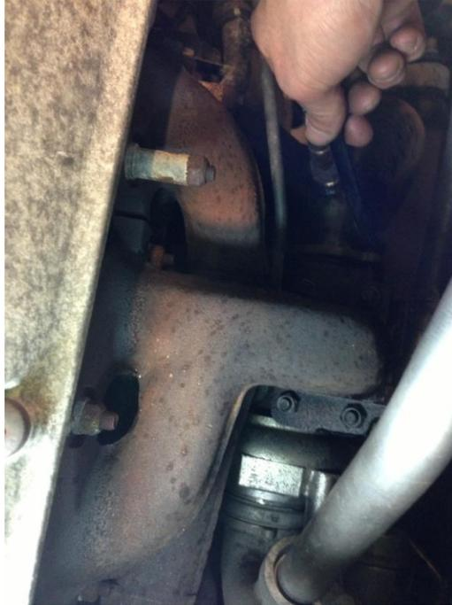
3. Next generously soak the bolts holding the downpipe to the cat back exhaust section (this particular car already had an aftermarket exhaust which was replaced with a Krona Performance Turbo back ☺)
