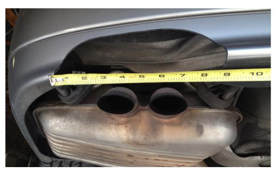
18. Once you have made the bumper modification you should now be getting excited... You are almost done:-)! You may now install the muffler/tip section, be sure to slip a clamp over the under axle pipe prior to making the connection. Lift the muffler into place and install the hangers in the factory location.
