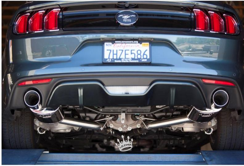
You should have a minimum of a ¼" gap between the exhaust and body to allow for thermal expansion as the system heat cycles.
