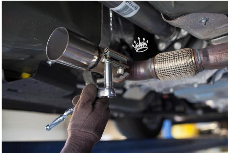
2. Slide the supplied 3" band clamp over the adapter section and then install the 3" to dual 2.5" krona mid pipe. Do not tighten the 3" clamp as it this time just ensure it is on your exhaust assembly.
