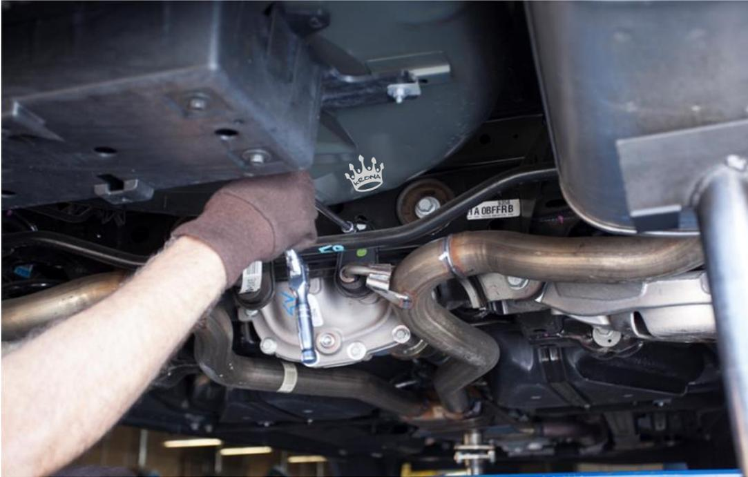
5. Place a support under the factory center resonator and now loosen the factory band clamp (x2 15mm bolts) attaching the downpipe to the mid pipe/resonator.
