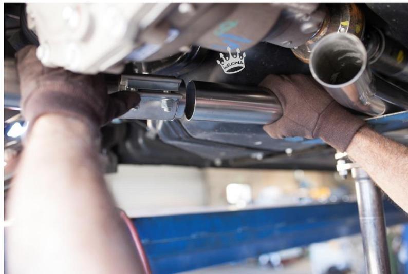
6. With both sides installed equally adjust the distance between the connections using the clamps. Do tighten at this time.
