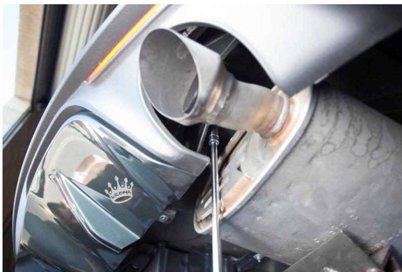
4. Next you may remove the factory rear exhaust hangers holding the system to the rear suspension just above the differential cover(x1 13mm bolt each side). These hangers can remain on the system until it is removed from the vehicle. Spray some lubricant on the rubber portions as you will need to remove these and reinstall on your new Krona system.
