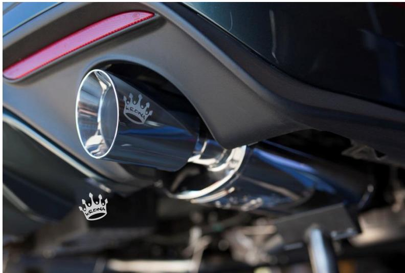
8. When tightening down all bolts and clamps working your way forward it is important to also ensure all piping is parallel to the ground. This indicates proper fitment has been achieved.
