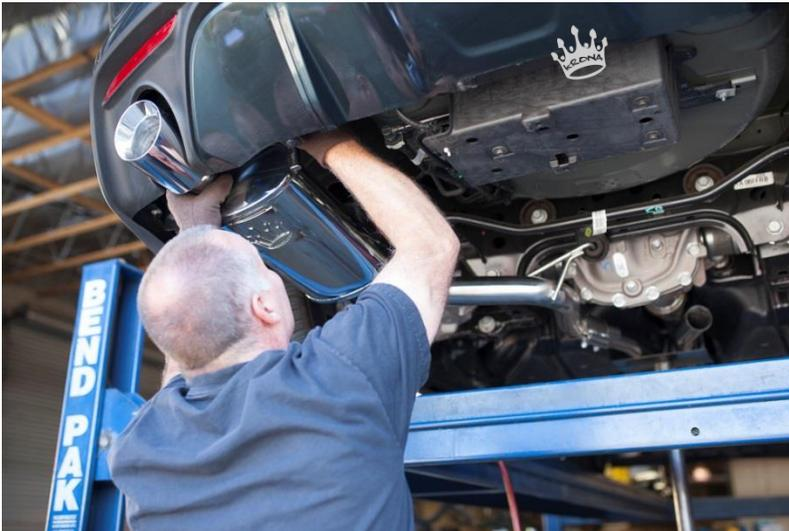
5. Slide your mid pipe back to allow for roughly a ½” gap between the connecting pipe sections. The clamp may be installed but do not tighten down at this time.
